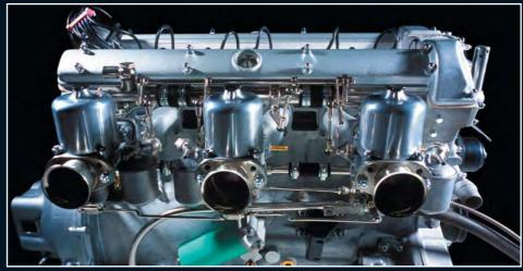
based around a new 4 bolt block, forged rods, steel crank, Cosworth pistons, big valves and special cams.
